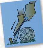
Brace the ax head on the ground between two wooden pegs or tent stakes and a log about 6 inches in diameter. Another Scout can help hold the ax steady. Place the file on the edge of the blade and push it into the bit. Use enough pressure so that you feel the file cutting the ax metal.
